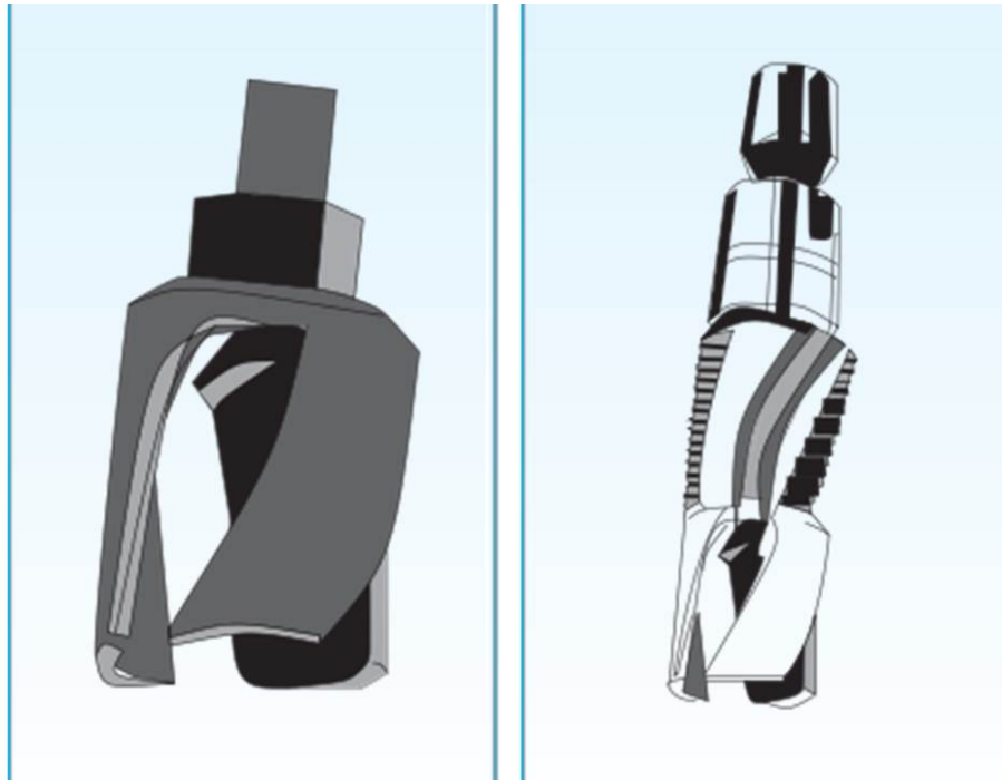
Figure 15 - Two Acceptable Slotted Core-Cutters. The cutter on the right is a combined cutter-tap
