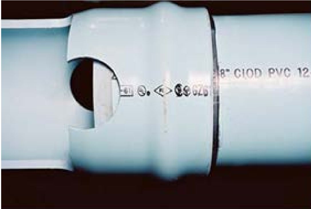
Figure 7 - Properly inserted pipe joint with cut-away
